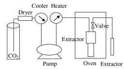
Fig. 1. Schematic diagram of supercritical extraction apparatus
