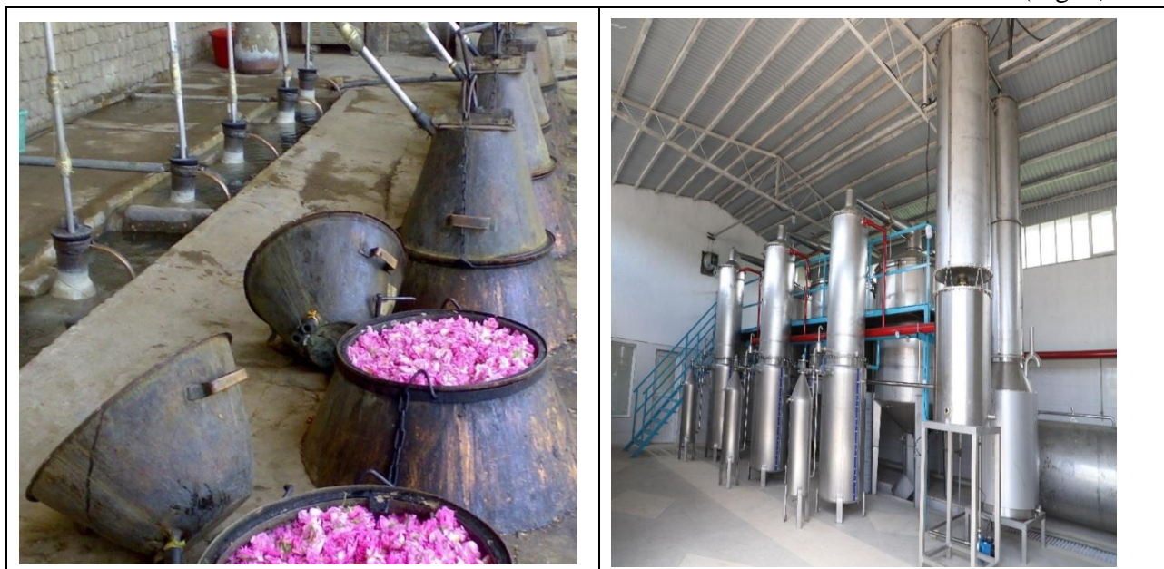
Fig. 1. The production of Rose water in the Traditional way (left hand), and industrial way (right hand)
