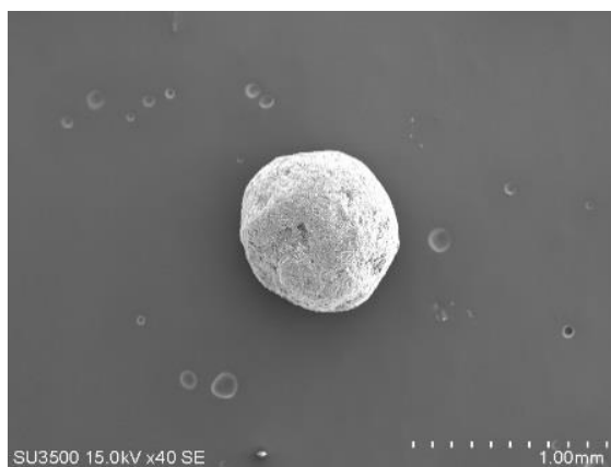
Fig. 1. SEM micrograph of the optimized pellet ( \times 40 )
