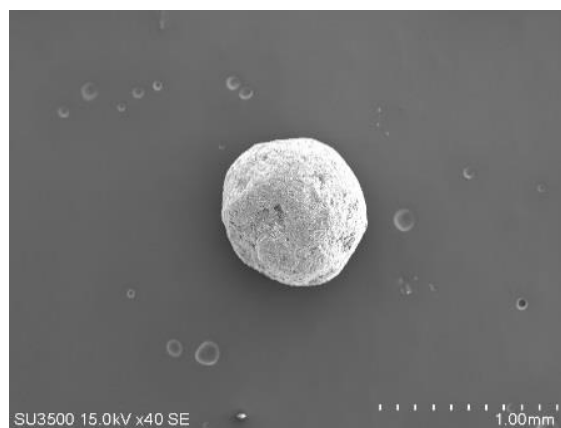
Fig. 1. SEM micrograph of the optimized pellet ( \times 40 )
