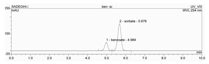
Fig. 1 - Illustrates the chromatogram of a standard solution, which contains 40 mg  $\Gamma^1$  of Sodium benzoate and 4 mg  $\Gamma^1$  of Potassium sorbate
