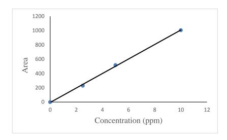
Figure 1- Calibration curve of rutin at 350 nm wavelength.
