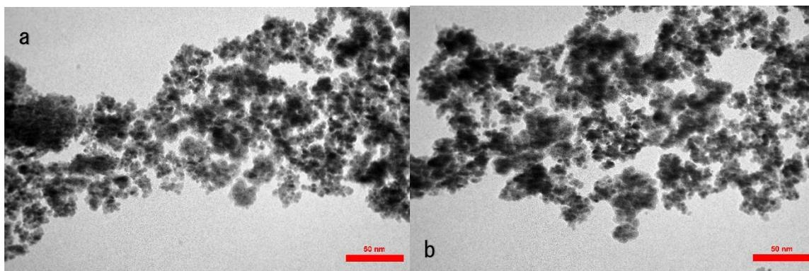
**Fig. 2.** TEM image of the colloidal INPs synthesized using fenugreek seeds extract in the optimal condition (extract to iron salt volume ratio of 1.5, incubation time of 90 min, and temperature of 36.5 °C)
