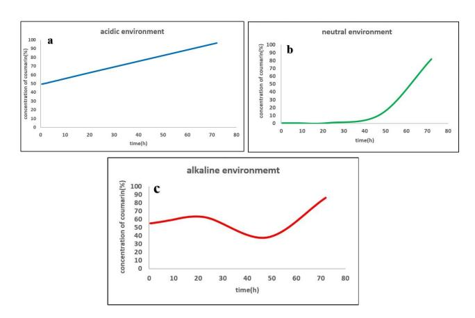
**Fig. 6.** Release profiles: a) in an acidic, b) in a neutral, and c) in alkaline conditions from nano-encapsulated coumarincontaining electrospun nanofibers.
