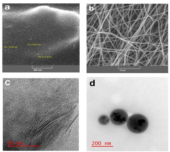
**Fig. 4.** SEM examination of coumarin encapsulated in nanoscale carriers (a), electrospun fibrous mats consisting of 10 % nano-capsule-loaded coumarin (b), and high-resolution TEM images of electrospun fibers containing nanoencapsulated coumarin (c and d).
