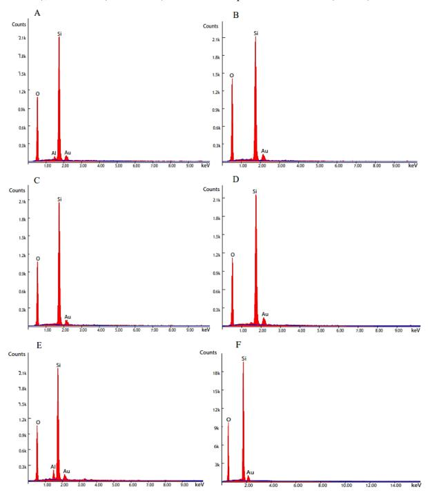
**Fig. 7.** Analysis of silica purity in some *Equisetum arvense* populations with energy-dispersive X-ray spectroscopy. A: Irde-Mousa (*EAP1*), B: Sarab (*EAP4*), C: Kandovan (*EAP5*), D: Tunnel-e-Kandovan (*EAP6*), E: Takor (*EAP7*), F: Marzanabad (*EAP11*).
