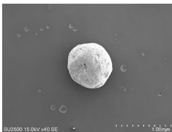
Fig. 1. SEM micrograph of the optimized pellet ( \times 40 )
